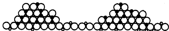
Fig. 5.—Possible structure of supported chromic oxide on aluminum oxide: O, O^{2-} ; o, Al^{+3} ; ●, Cr^{+3} .
